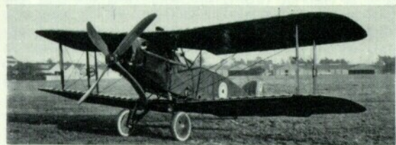
Left: Single-bay wings of 30 ft. 11½ in. span, 7 ft. chord and an aspect ratio of 4.69 were fitted first to A7860 (R.A.F. 4d engine). The Falcon-powered F.2B F4360 is here seen at the R.A.E., Farnborough, on 25th January 1923, fitted with similar wings. (Photo: Crown copyright); Right: Also photographed on 25th January 1923 was F4728, fitted with the experimental three-bay wings of aspect ratio 9.78. (Photo: Crown copyright)
