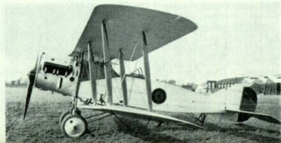
Above: Possibly a SABCA-built Bristol F.2B, this was No. 45 of l'Aeronautique Militaire Belge, with 300-h.p. Hispano-Suiza engine, oleo undercarriage and horn-balanced rudder. Below: One of twelve new-built Bristols supplied to Spain in 1924 with 300-h.p. Hispano-Suiza, oleo undercarriage and Frise ailerons.
