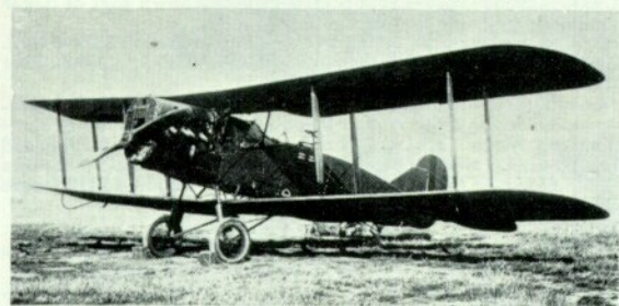
Above: Possibly a SABCA-built Bristol F.2B, this was No. 45 of l'Aeronautique Militaire Belge, with 300-h.p. Hispano-Suiza engine, oleo undercarriage and horn-balanced rudder. Below: One of twelve new-built Bristols supplied to Spain in 1924 with 300-h.p. Hispano-Suiza, oleo undercarriage and Frise ailerons.
