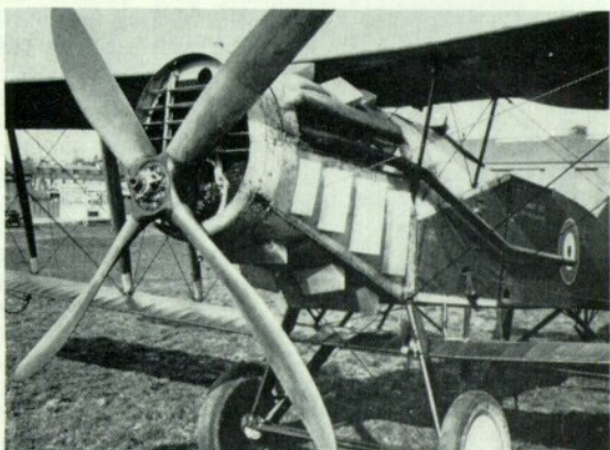
Above: Post-war use of the Bristol F.2B in India and the Middle East led to cooling problems that were investigated at Farnborough. One attempted solution was this liberally-louved cowl, almost certainly on C4654, photographed on 29th April 1923. (Photo: Crown copyright); Below: The greatly enlarged upper fin and rudder fitted in 1920 to the Puma-powered Bristol Fighter C4655 were similar in outline to the original surfaces. At Farnborough a few years later C4776 was fitted with revised vertical surfaces incorporating a balanced rudder, foreshadowing the tail unit of the Bristol Fighter Mk. IV. This photograph is dated 23rd March 1925.
